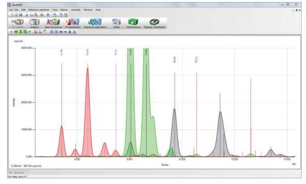
QuantEZ® software, coupled with the high-resolution SDD, provides an easy-to-use qualitative evaluation of spectra. Shown are overlapped spectra with element line markers.
