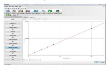
An Illustration of an empirical calibration curve is shown, one of the flow bar steps to set up an application.
