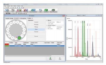
EZ Analysis interface, available in various languages, is used for routine measurements. A live spectral display is shown in the window on the right.
