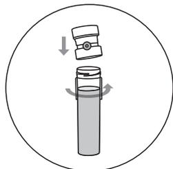
Screw the **DigFILTER** (using the end with the plug) onto a 50 ml **DigTUBE** containing a cooled sample.
