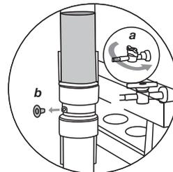
Open the valve and remove the plug from the opposite port.
