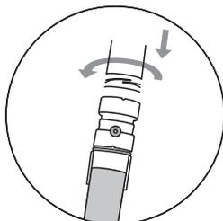
Screw a clean **DigTUBE** onto the opposite end of the **DigFILTER**.
