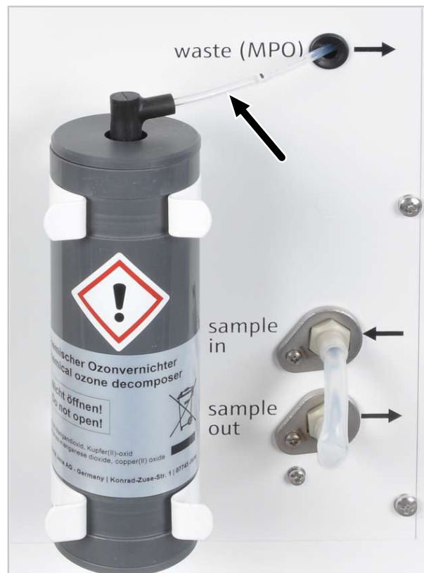
Figure 73 Replacing the chemical ozone decomposer
