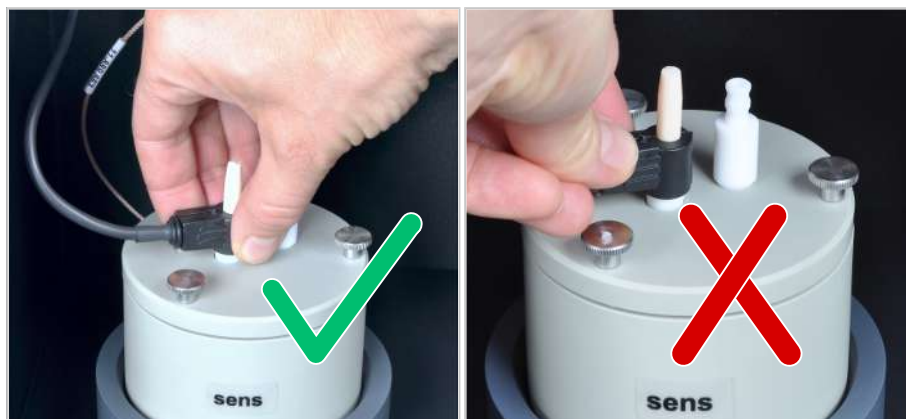
Figure 72 Correct handling of the combined electrode
