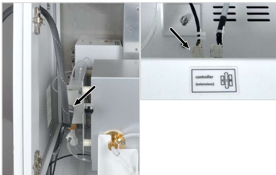
Figure 42 Connection of the gas transfer line in the basic module
