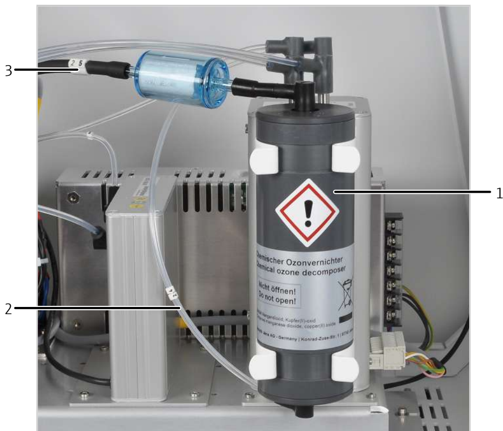
Figure 70 Replacing the chemical ozone decomposer
