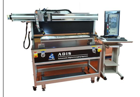
**Hardware:** The main frame is made of lightweight aluminum profiles The single LED light source also allows the CSS to be extremely compact and easily transferable.
